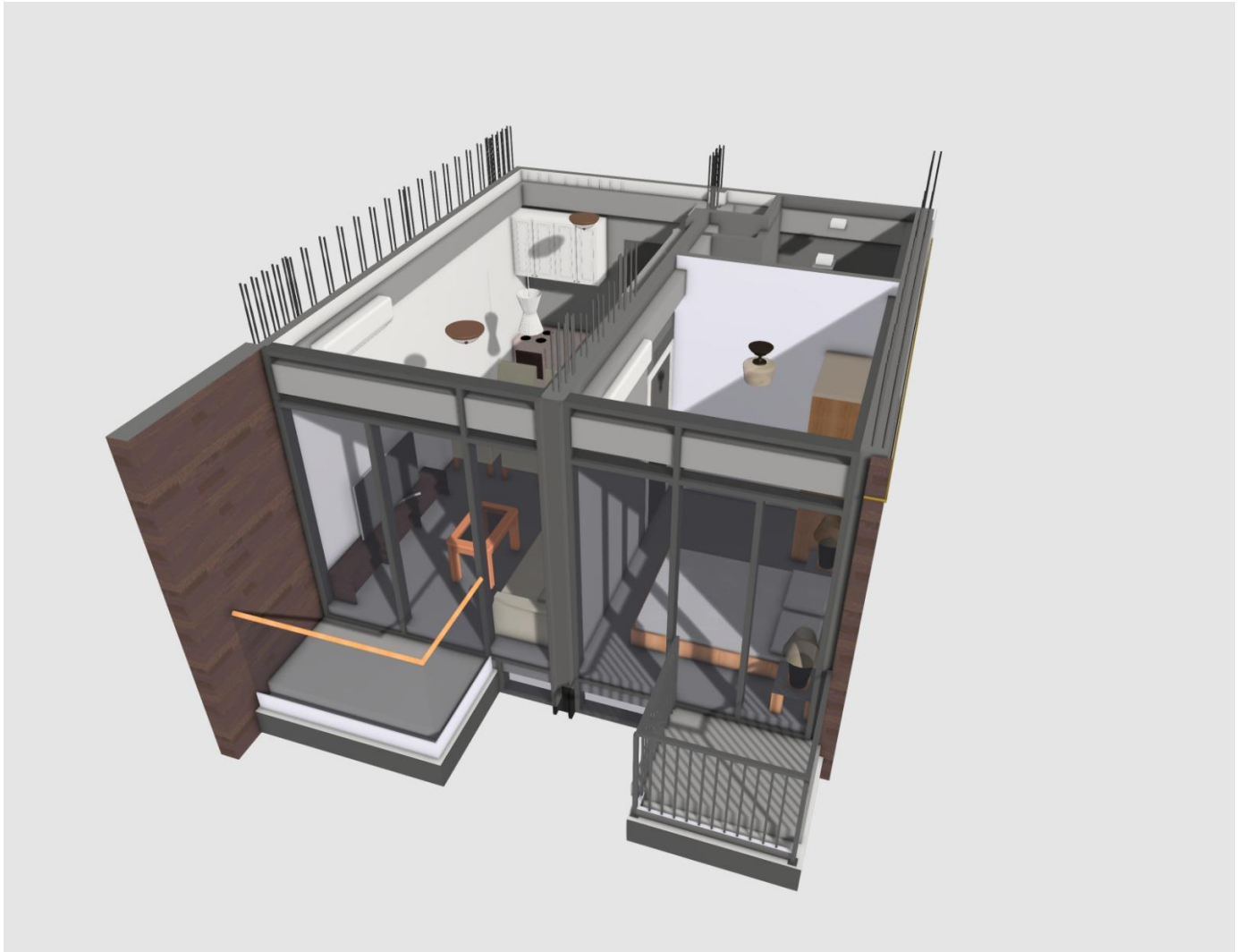
BIM model of a “5-face module 2-bedroom unit” built with concrete MiC developed by Chun Wo and P&T
